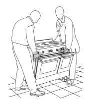
Figure 6 Correctly raising the cooker
